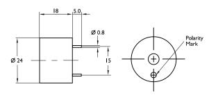
Dimensions : Millimetres Tolerance: ±0.5mm
