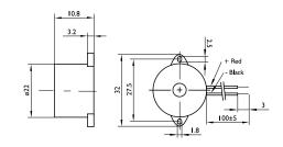
Dimensions : Millimetres Tolerance: ±0.5mm
