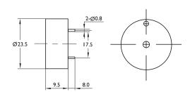
Dimensions : Millimetres Tolerance: ±0.5mm
