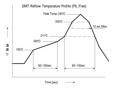
Note: 245 is Less than 15 sec. ,but only pass the lead free reflow once. The SPL should be in ±4dB compared with initial one, Higher than 81 dB.
