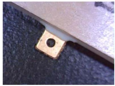
PIN bottom are not allowed to overflow glue, glue over the top criteria: Max.0.25mm PIN 底面不允許有溢膠,上面溢膠標準:Max.0.25mm
